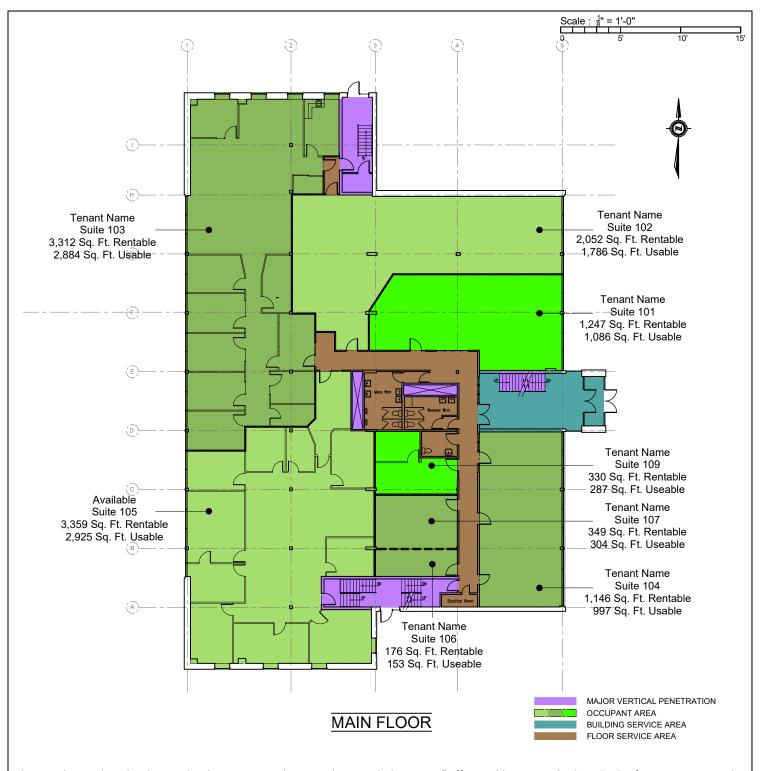
The unit depicted on this drawing has been measured in accordance with the BOMA "Office Buildings: Standard Methods of Measurement and Calculating Useable Area (ANSI/BOMA Z65.1-2010)", Method A (Legacy Method), within the limits of accuracy imposed by site conditions.
